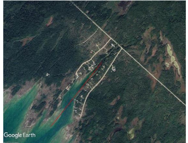
Figure 7. Baptist Harbour. The red line indicates the length L (1100 metres) used in equation (v).
