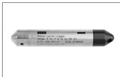
Figure 16. Onset Hobo U-20 water pressure and temperature logger.
